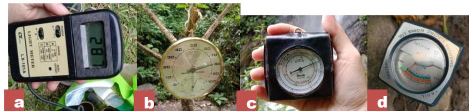
Gambar 1. a) light meter, b) hygrometer, c) altimeter, d) soil tester
