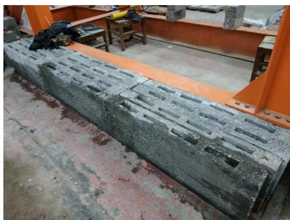
**Gambar 1.** Benda Uji Dinding Panel Beton *Styrofoam* Berlubang
