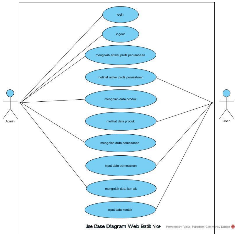
Gambar 1. Use Case Diagram Batik Nice 1
