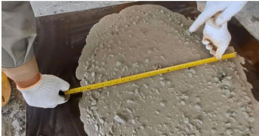
Gambar 1. Uji Slump Flow
