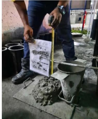
Gambar 4. Test Slump
