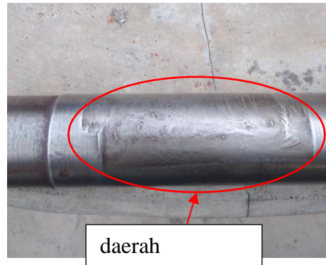
Gambar 15. Foto makro permukaan selimut poros as
