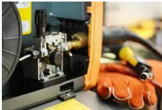
Gambar 9. Motor wire feeder
