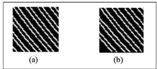
Gambar 3.b. Citra batik geometri (a)segmentasi *canny detection* (b)*canny detection* dan *thresholding otsu*
