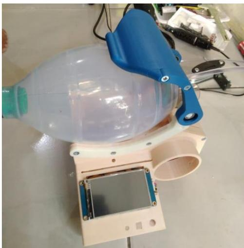
Gambar 7 Ventilator mekanik
